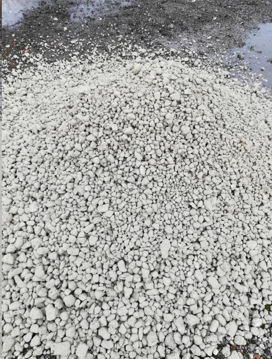
*Figure 24: 10-32 fraction screened before separation*
