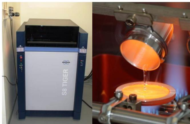
Photograph 6: XRF device (left) on fused bead (right)
