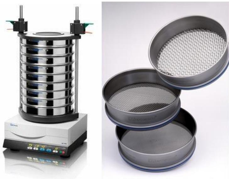
Figure 2 : particle size composition test device
