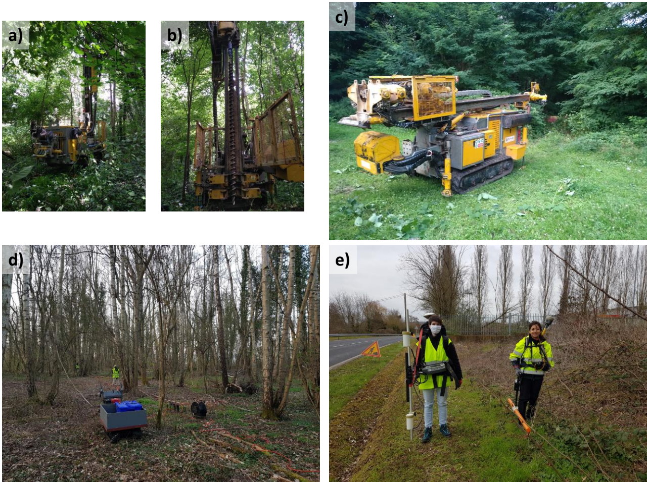
Figure 6 : a), b) and c) light core drill used on site to dig the 4 boreholes FP1 to FP4. d) Light crawler wheelbarrow used to carry geophysical material (batteries and cables) on site; e) Geophysical tool used on site carried out manually at the North entrance of the site (see Figure 1).
