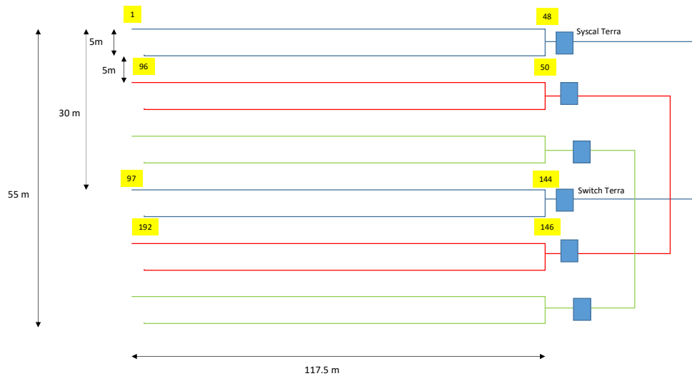
ERT configuration for the 3D survey
