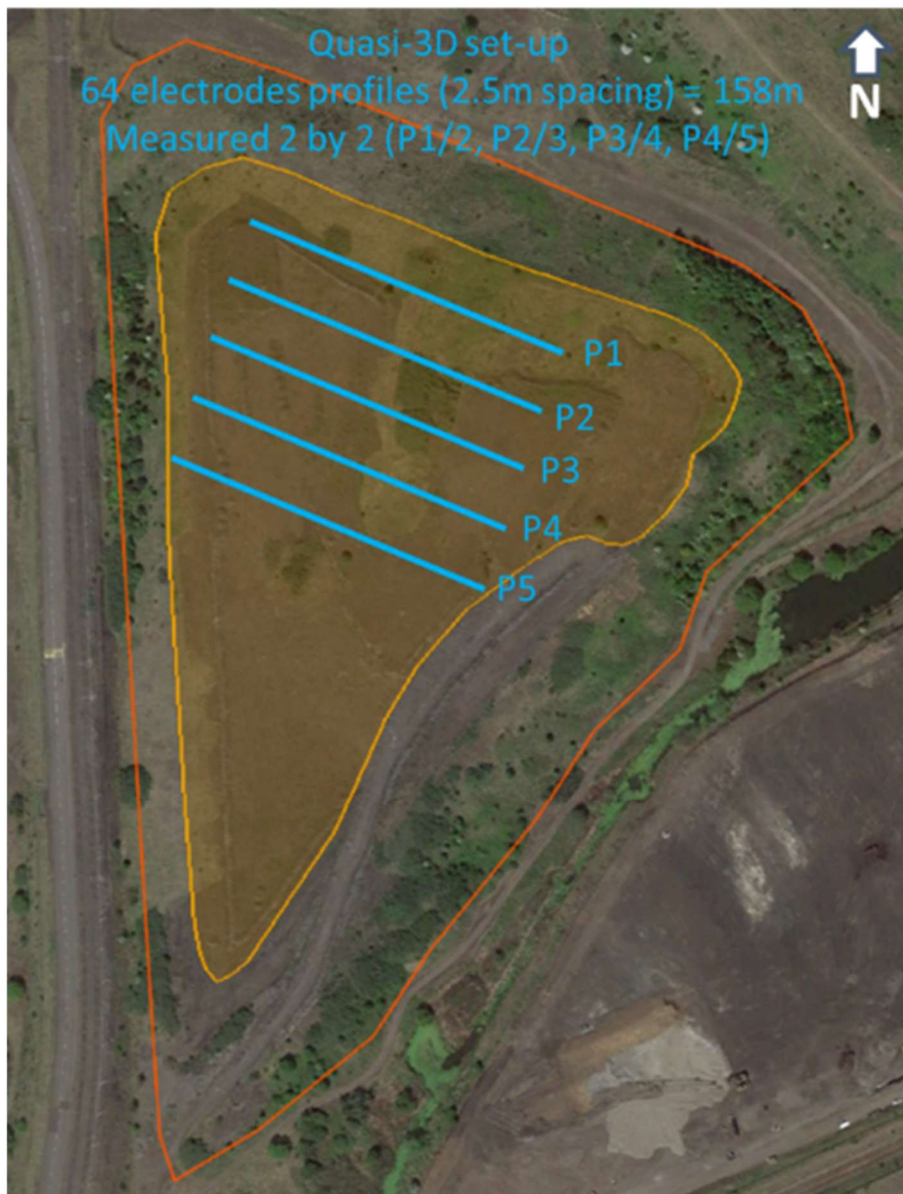
Figure 5 – example of 3D ERT/IP set-up (Electrical Resistivity Tomography and Induced Polarisation). In this example, first profile P1 and P2 will be measured simultaneously. Then, P1 is moved to P3 location to proceed the second measurement, and so on until P4/P5 profiles are measured. Their location would be defined according to EMI and Mag survey.
