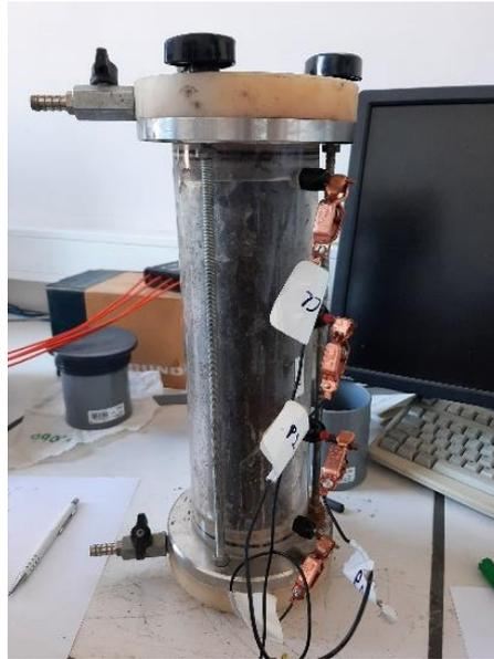
Figure 3: Column were the lab measurements of ERT, IP and SIP were carried out. The columns have a volume of 1.5 dm<sup>3</sup>, a diameter of 8 cm and height of 30 cm.
