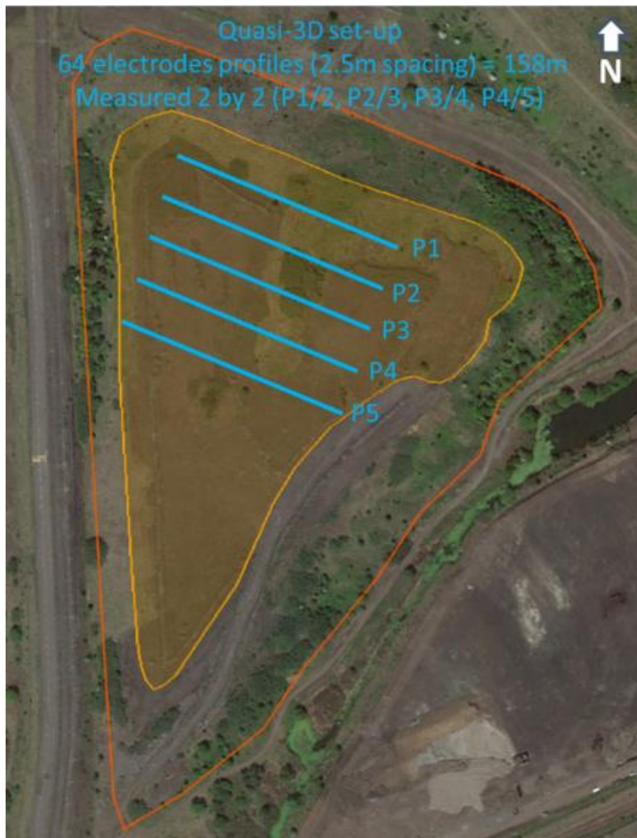
Figure 7. Example of 3D ERT/IP set-up (Electrical Resistivity Tomography and Induced Polarisation).
