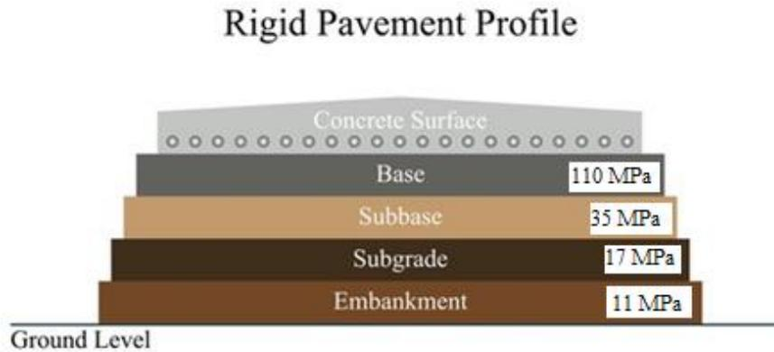
Figure 2: Minimal bearing capacity values for a use in road construction in Wallonia (according to “Qualiroutes” criteria)
