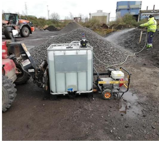
Picture 7: Equipment used to spray acetic acid reagent
