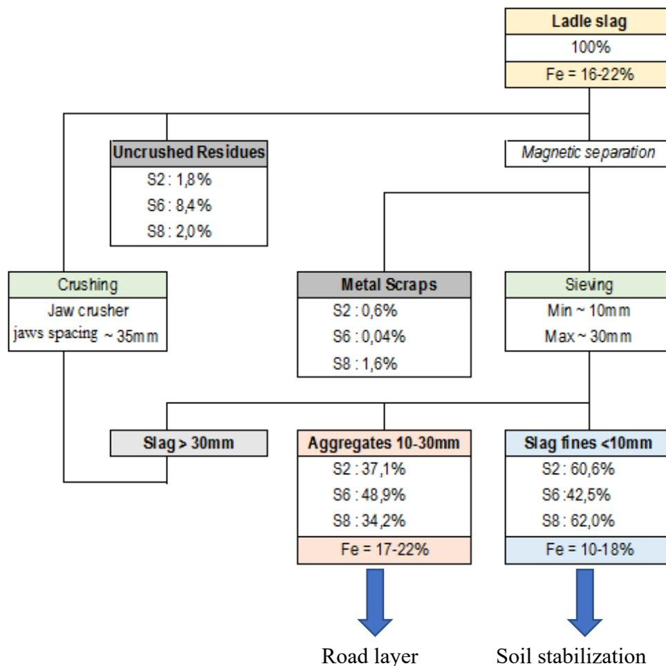
Figure 1 : Flowsheet of the slag sample processed in CTP
