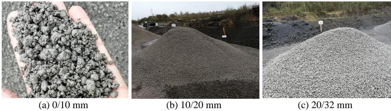
Picture 9 : Slag fractions obtained by sieving
