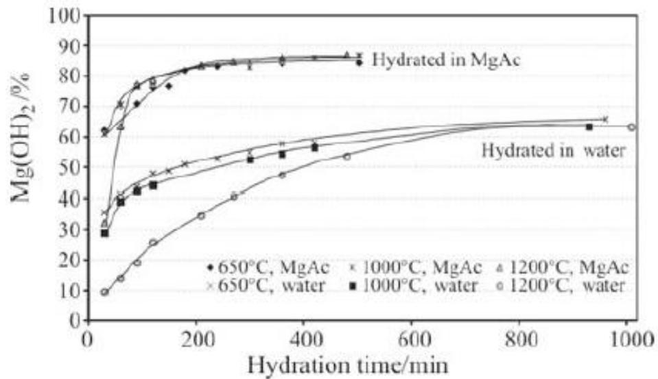
Figure 6 : Effect of acetate ions addition on the hydration rate of MgO
