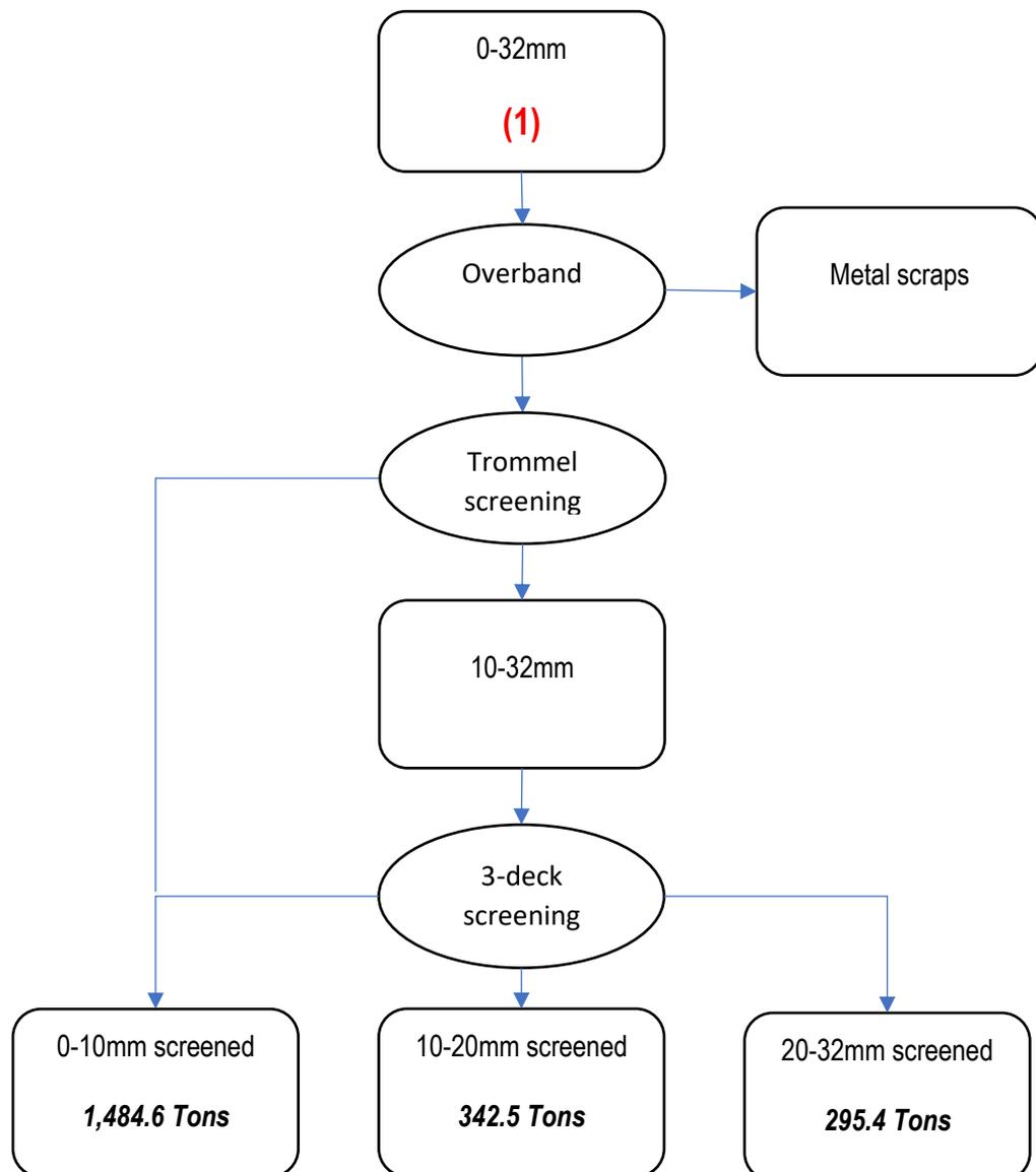
Figure 3: Process flowsheet – Treatment of the sieved 0/32 mm fraction in order to produce three sub-fractions: 0/10 mm, 10-20 mm and 20/32 mm
