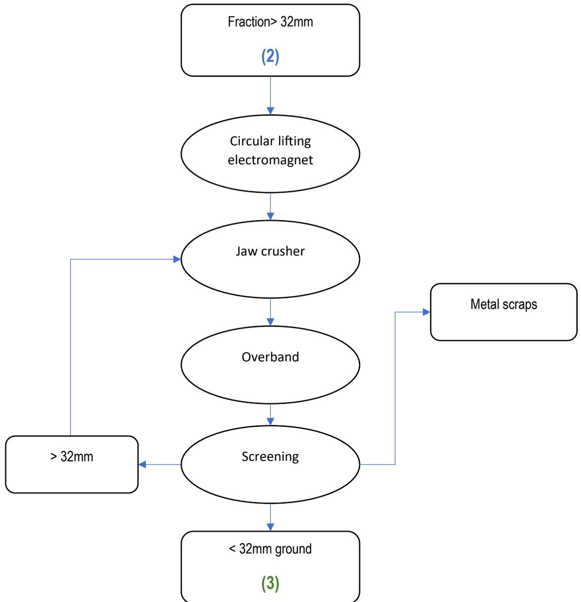
Figure 4: Process flowsheet – treatment of the sieved fraction > 32 mm to reduce its grain size below 32 mm
