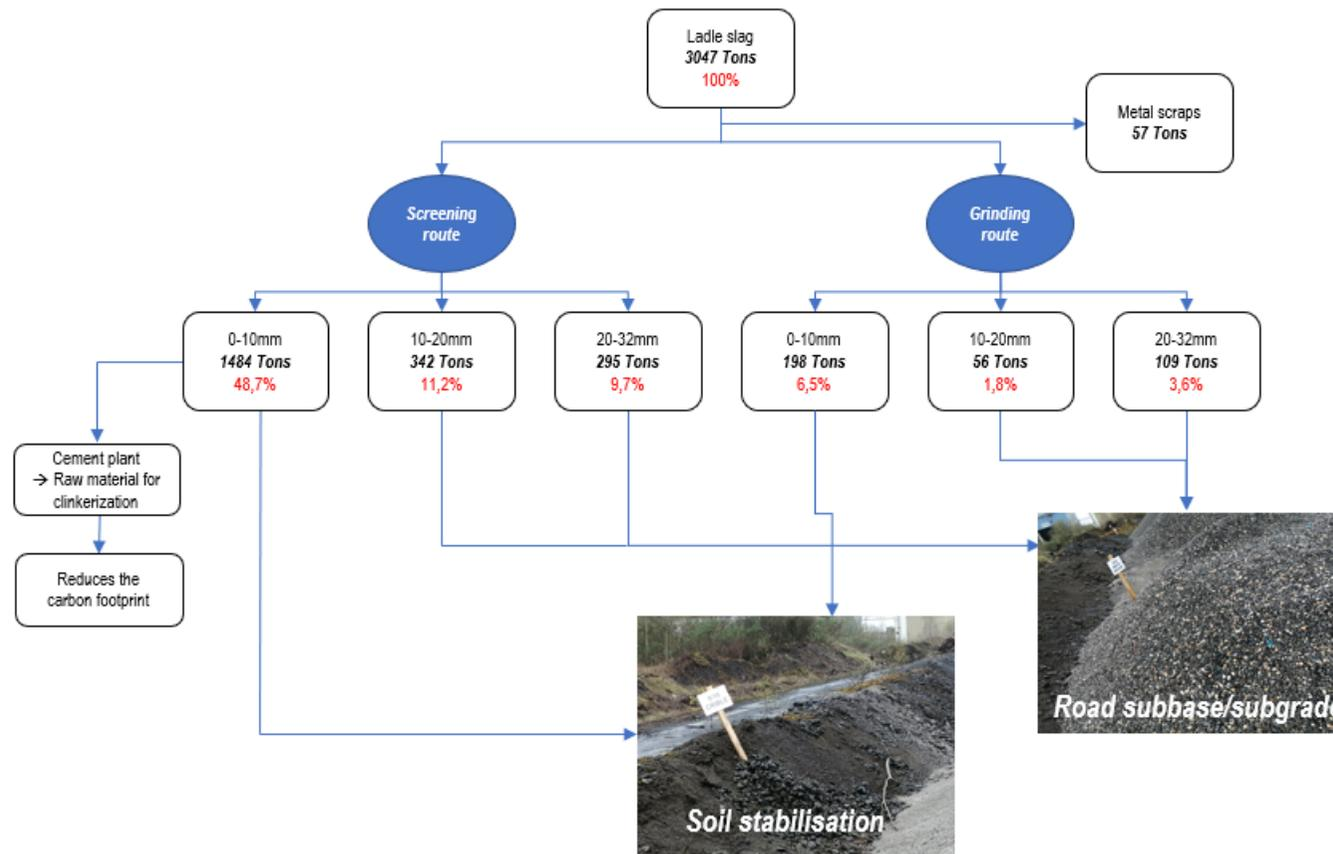
Figure 7: Global matter recovery resulting from on-site slag processing
