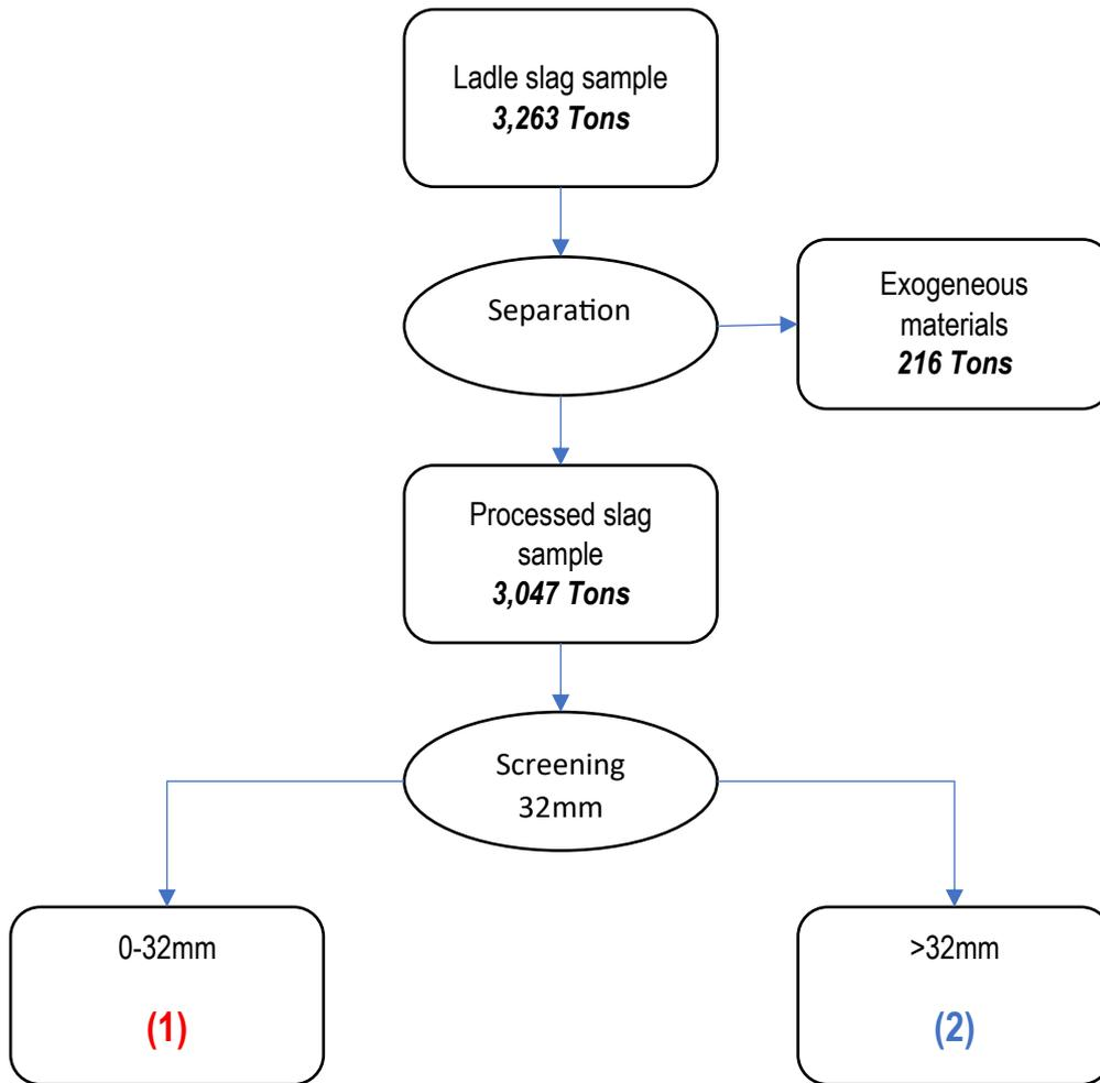
Figure 2: Process flowsheet - production of 0/32 mm and > 32 mm slag fractions
