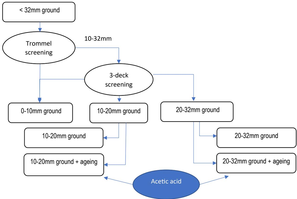
Figure 5 : Process flowsheet - Treatment of the ground 0/32 mm fraction in order to produce three sub-fractions: 0/10 mm, 10-20 mm and 20/32 mm
