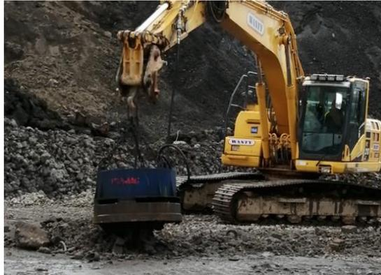
Picture 5: Circular lifting electromagnet
