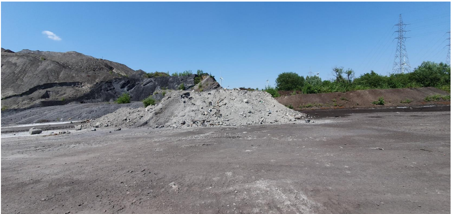
Figure 5 : Slag directly removed - too many exogenous material
