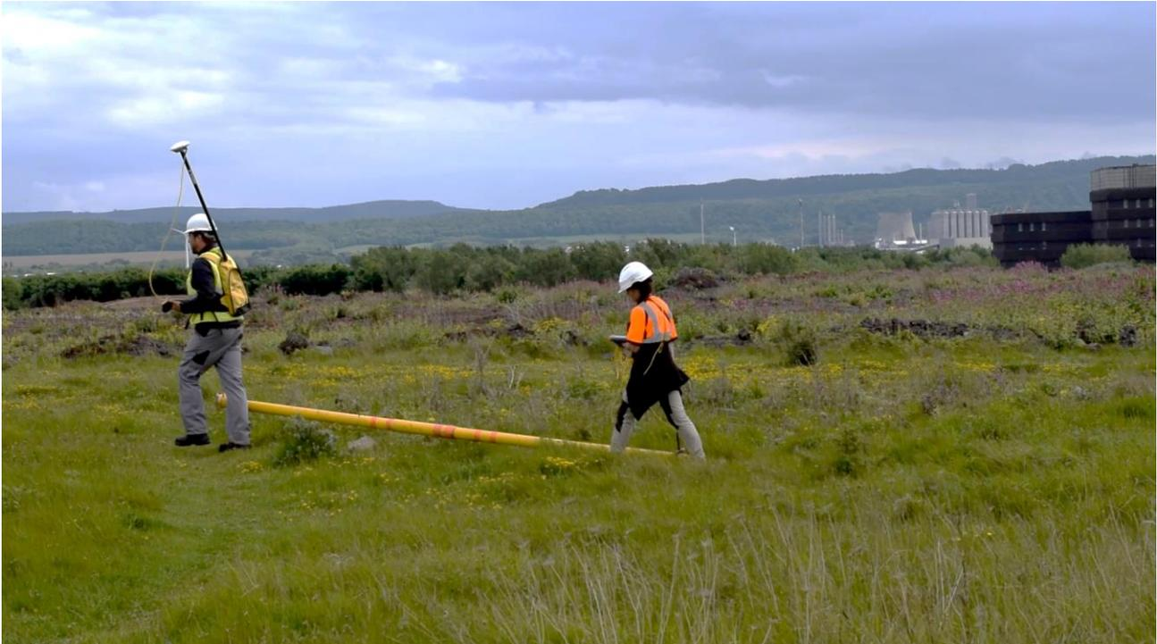
*Figure 15 : photography of the DUALEM421S tool on Teesside site*
