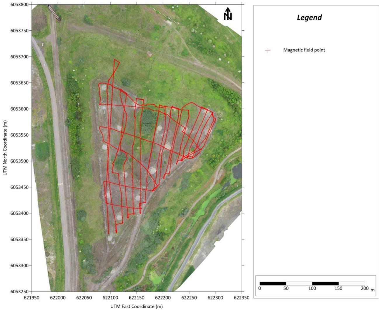
Figure 10 : Magnetic field measurements points map with Geometrics G858 magnetometer
