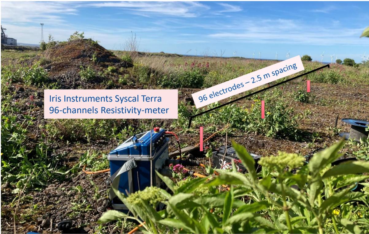
Figure 23 : Photo of the Syscal Terra equipment used for the Electrical Resistivity and IP Tomography survey
