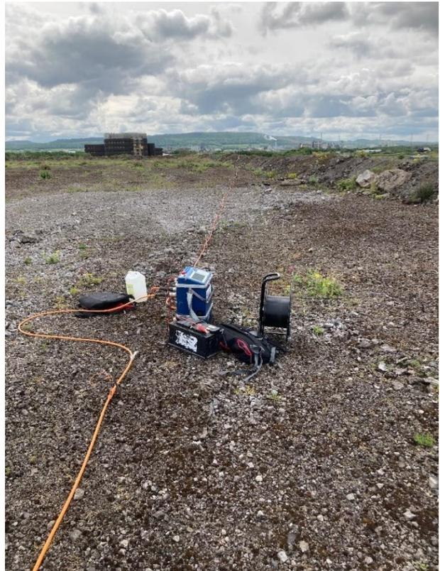
Figure 24 : Photographies of the ERT equipment on the Teesside site, in a vegetated area (left) and on a coarse-grained material (right)
