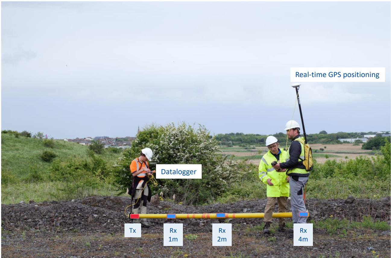
Figure 16 : Schematic details of the DUALEM421S tool
