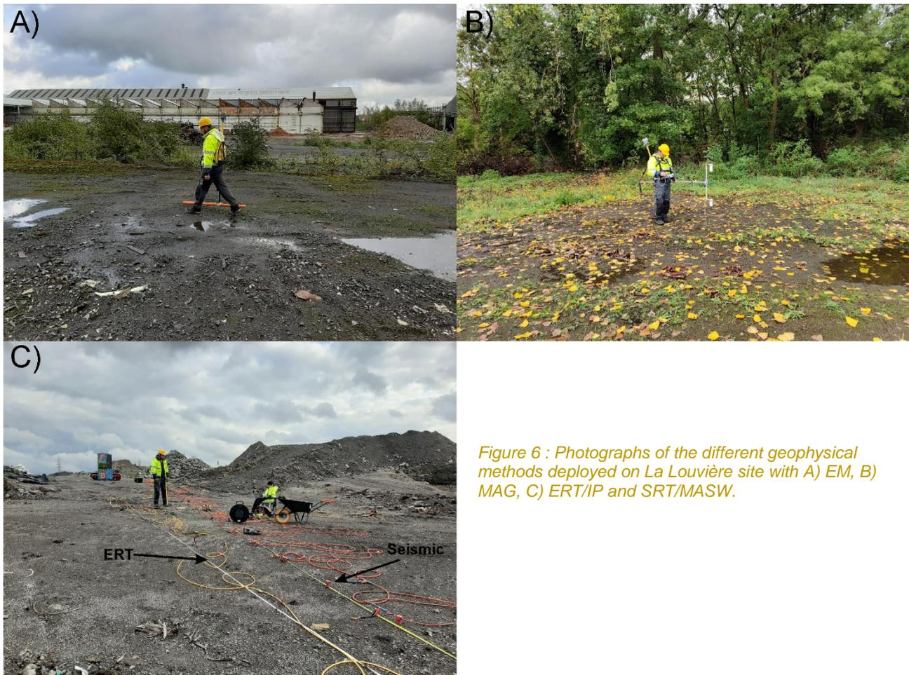
Figure 6 : Photographs of the different geophysical methods deployed on La Louvière site with A) EM, B) MAG, C) ERT/IP and SRT/MASW.
