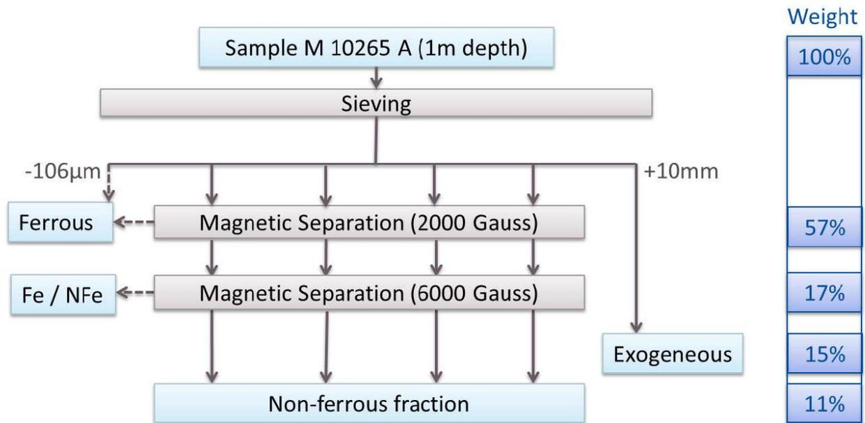
Figure 6: Example of mineral processing steps applied by CTP on sample from Pompey(1m depth) (from DT2.1.1)
