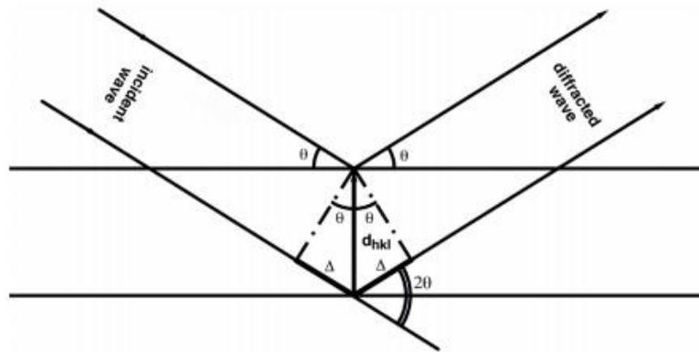
Figure 16- Bragg's representation of the diffraction condition (Lavina et al., 2014)
