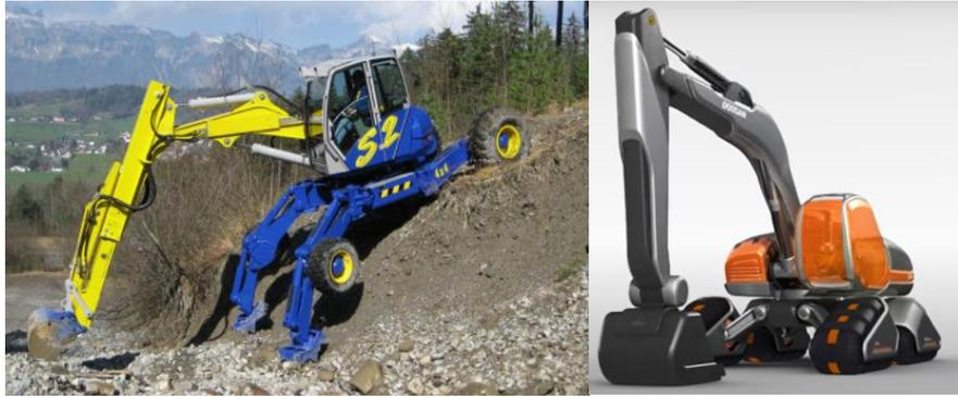
Figure 7- Walking excavator (left) (Kaiser, 2021) and excavator with four independent crawler tracks (right) (Doosan, 2010)
