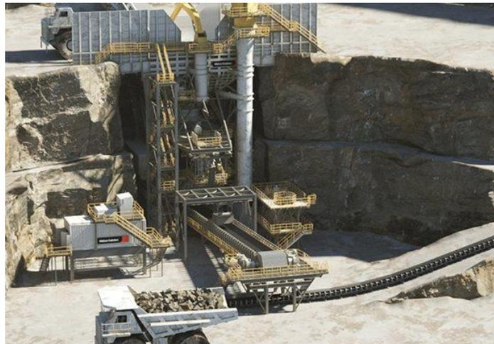
*Figure 39- Metso IPCC system (Metso Outotec, 2021a)*
