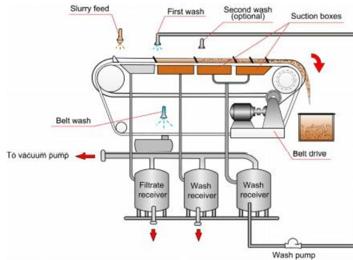
Figure 37- Horizontal belt filter (Wills & Finch, 2016)
