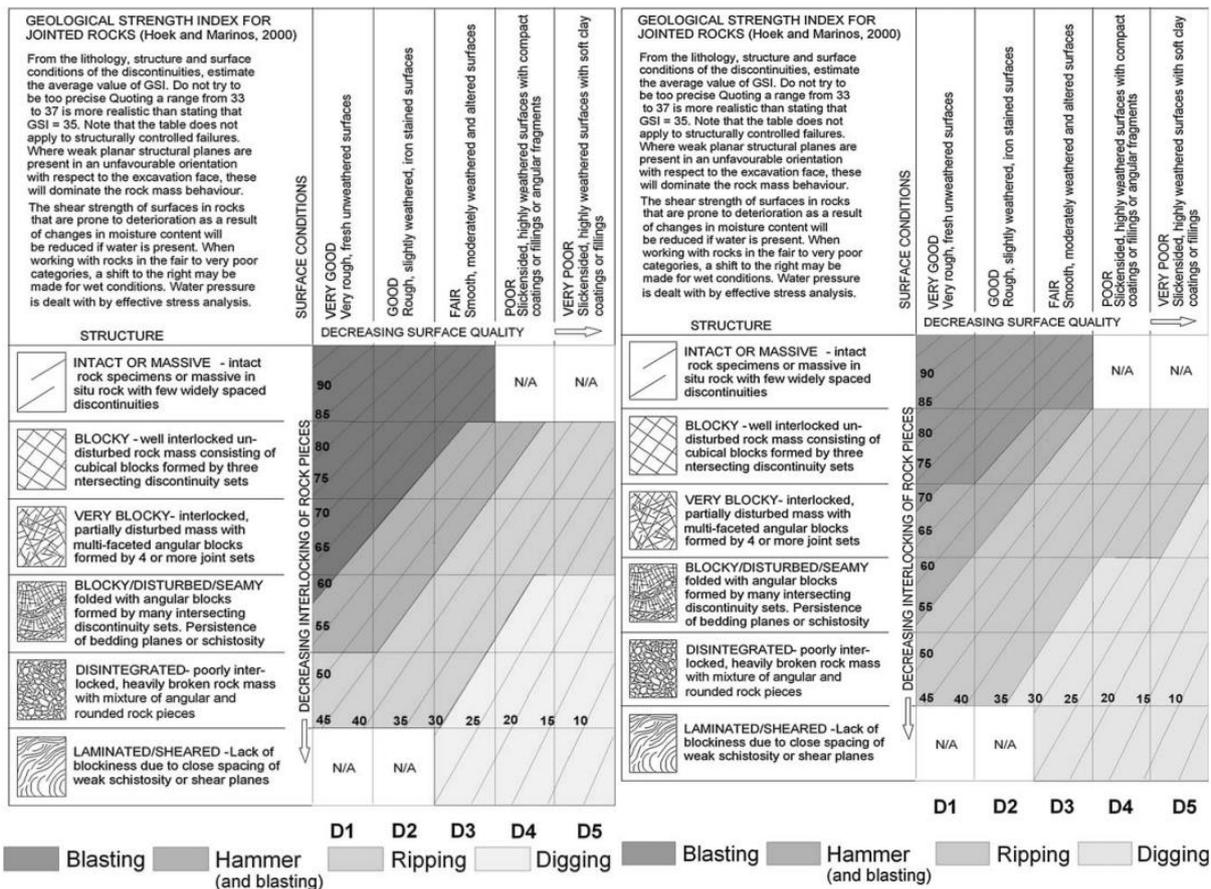
Figure 1- GSI chart for the assessment of excavatability of rock masses, left:  $I_{s50} \geq 3\text{MPa}$ , right:  $I_{s50} < 3\text{MPa}$  (Tsiambaos & Saroglou, 2010)
