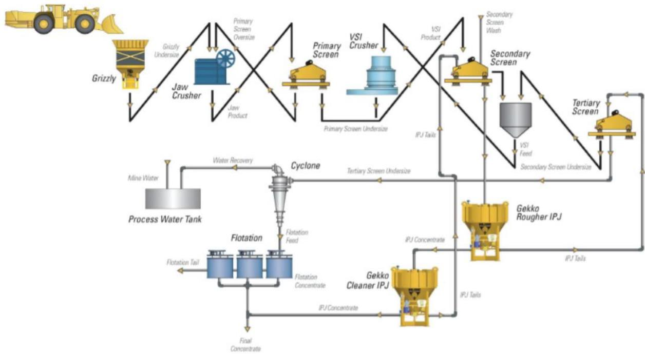
Figure 41- Process flow diagram for the Python plant (Dominy et al., 2010)
