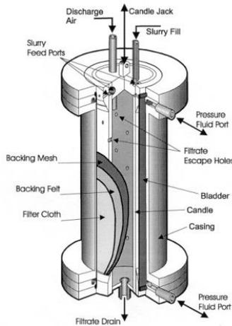
Figure 34- Tube press (Metso, 2015)
