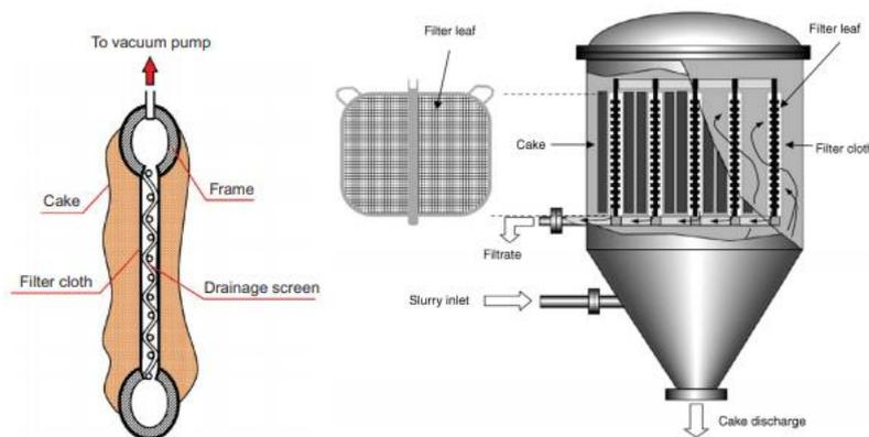
Figure 35- Left: cross section of a vertical leaf filter (Wills & Finch, 2016), right: sketch of a pressure leaf filter (Gupta & Yan, 2016)
