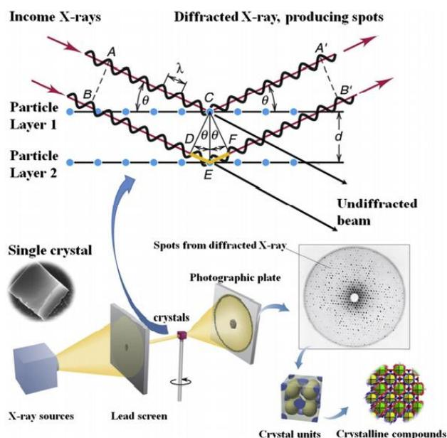
Figure 17- Schematic presentation of single crystal X-ray diffraction (Bashir & Liu, 2015)
