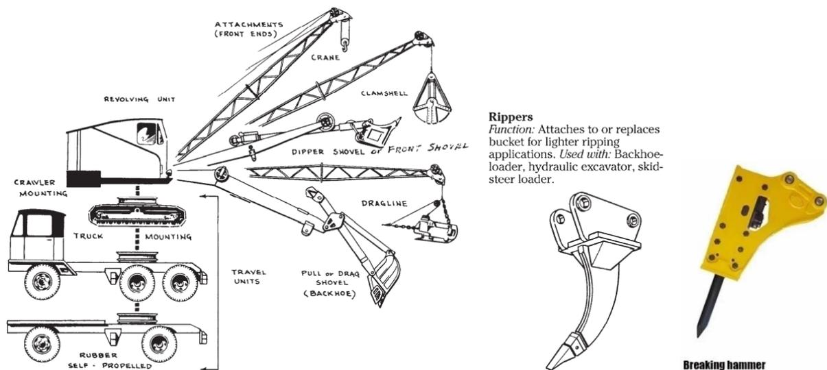
Figure 4- Attachments for hydraulic excavators (Nichols & Day, 2005)
