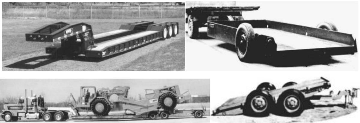
Figure 6- Top left : deck trailers, top right: low-bed semi-trailers, bottom left: loaded girder trailer, bottom right: tilt trailer (Nichols & Day, 2005)
