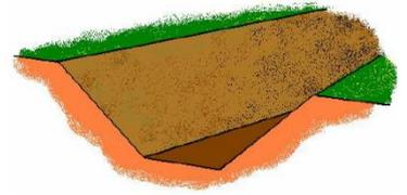
Figure B: Sloped trench (HMTRI, 2000).
