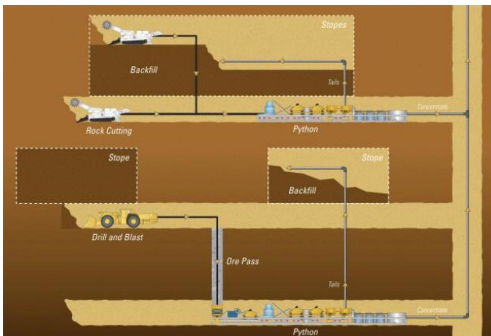
Figure 40- Underground processing concept based on the Gekko Python modular system (Dominy et al., 2010)
