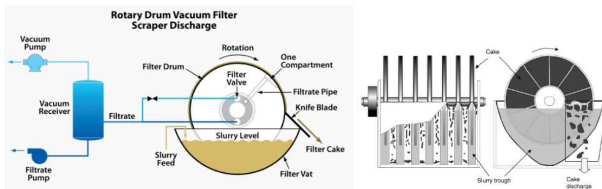
Figure 36- Left : rotary drum filter (Konline-Sanderson, 2021), right: schematic diagram of a disc filter (Gupta & Yan, 2016)
