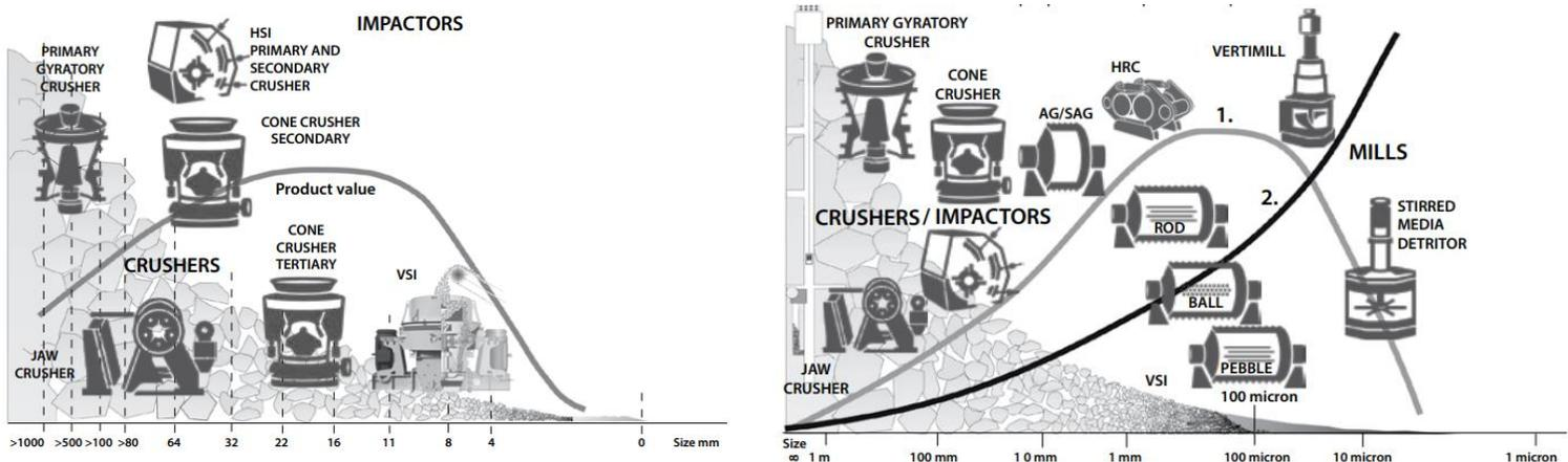
Figure 26- Left: crushing of rock and minerals, right: crushing and grinding of ore and minerals (Metso, 2015)
