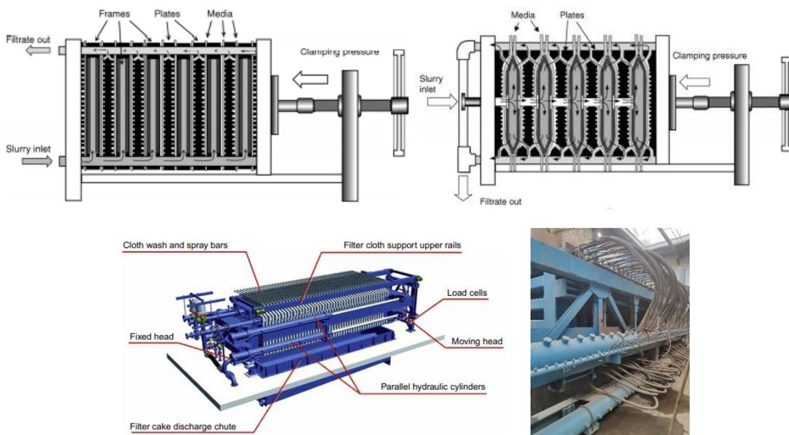
Figure 33- Above: left: plate and frame filter press, right: chamber press filter (Gupta & Yan, 2016). Below: left: horizontal pressure filter scheme (Wills & Finch, 2016), right: horizontal pressure filter picture, taken in the BIOTERRA NV plant
