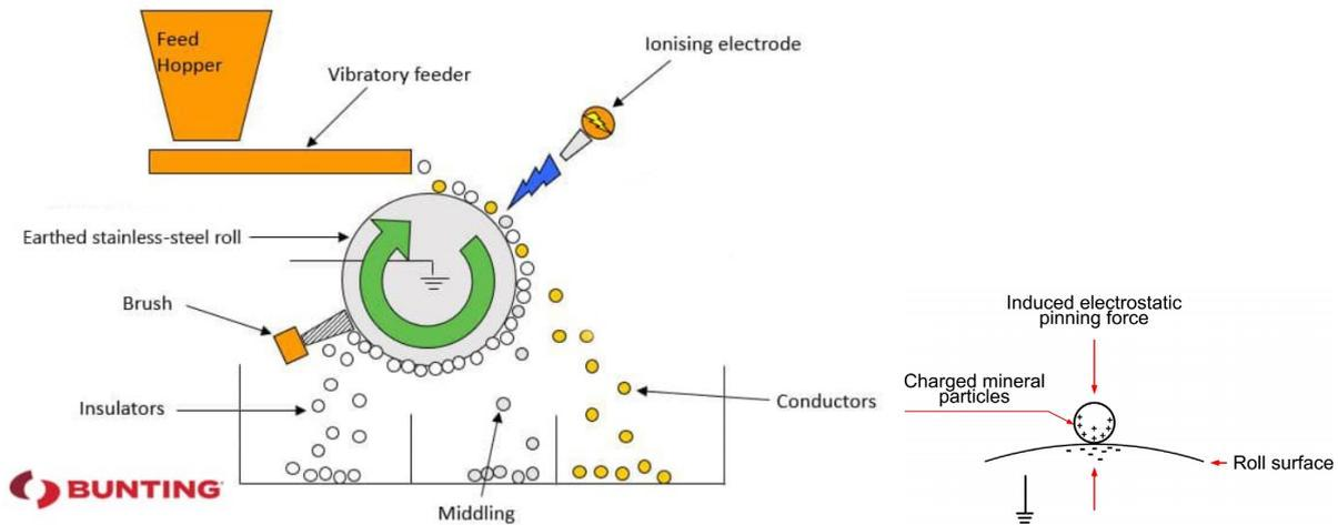
Figure 29- Left : Electrostatic separator (Fears, 2020) and right: representation of forces (Wills & Finch, 2016)
