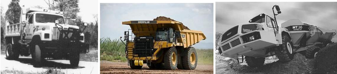
Figure 5- Left: on-highway dump truck (Nichols & Day, 2005), center: off-highway dump truck (Caterpillar, 2021a), right: articulated dump truck (Nichols & Day, 2005)
