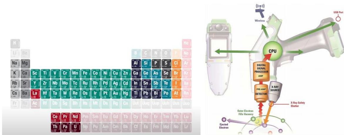
Figure 21- Left: General element range for EDXRF equipment (Hitachi, 2018), Right: Configuration of a typical handheld EDXRF-analyser (from Thermo Fisher (2021), cited by Analytical Committee (2019))
