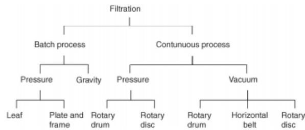
Figure 31- Classification of filtration processes (Gupta & Yan, 2016)
