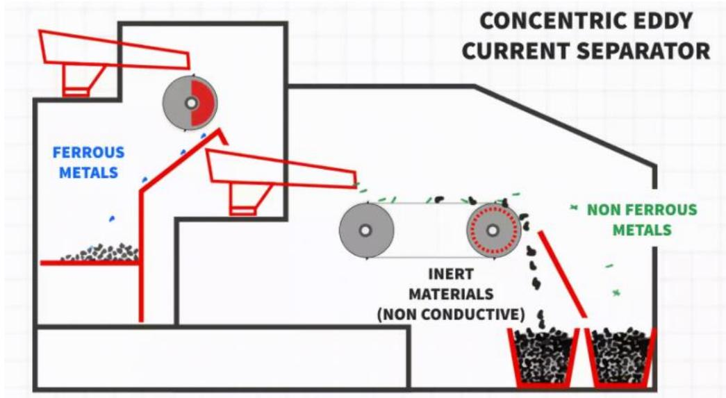
*Figure 28- Eddy current separator (Fears, 2020)*
