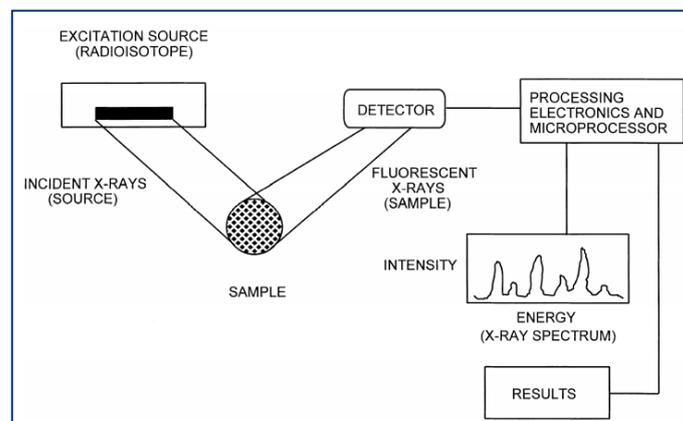
Figure 20- Block diagram of a typical (ED)XRF spectrometer (Kalnicky & Singhvi, 2001)
