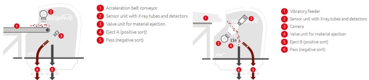
Figure 23- Functional principle of REDWAVE XRF 2-way belt type (left) and REDWAVE XRF/C 2-way free fall system (right) (REDWAVE, 2021h)
