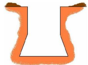
Figure D: Bellbottom pier whole trench (HMTRI, 2000).
