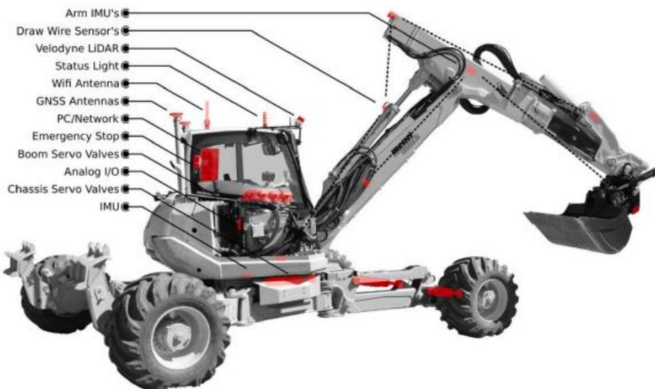
Figure 11- Extensive hardware changes and main components added to a standard walking excavator (Jud *et al.*, 2021)
