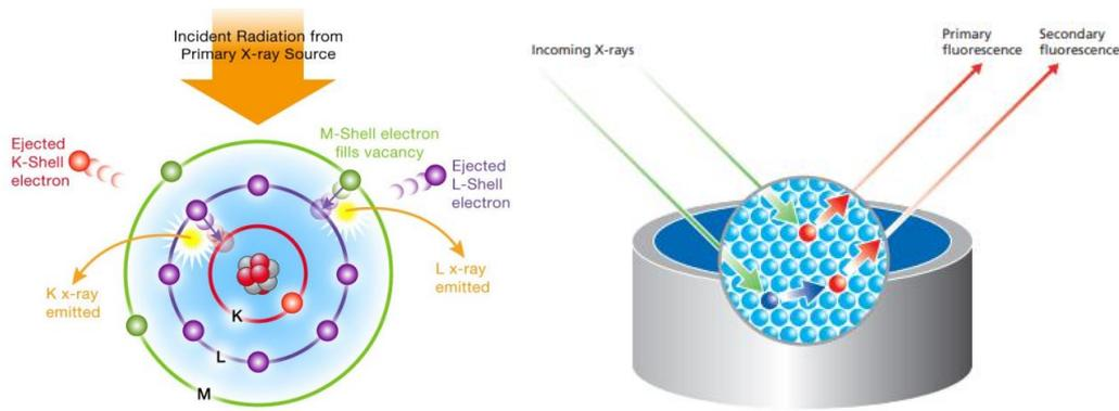
Figure 19- Left: X-ray fluorescence process (Yerly, 2014), right: primary and secondary fluorescence (Brouwer, 2010)
