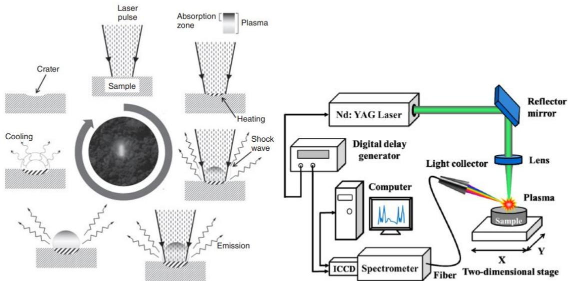
Figure 22- Left: Interaction between a solid surface and a laser pulse during a LIBS (Cremers et al., 2016), right: LIBS spectrometer device (Zou et al., 2014)
