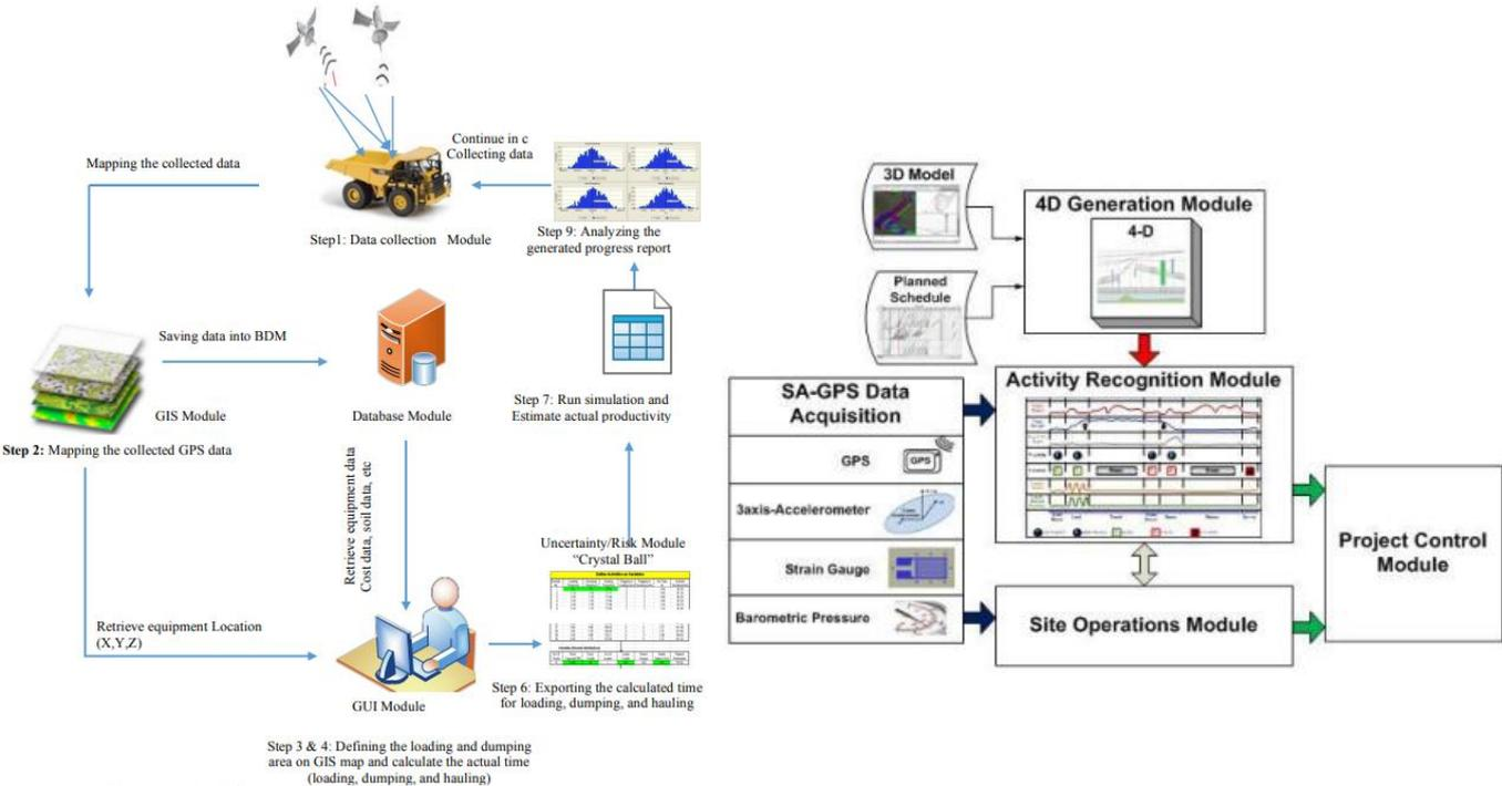
Figure 13- Left: non-vision based technologies relying only on GPS-data (Alshibani & Moselhi, 2016), right: non-vision based technologies relying on GPS-data coupled with a variety of sensors (Ibrahim & Moselhi, 2014)
