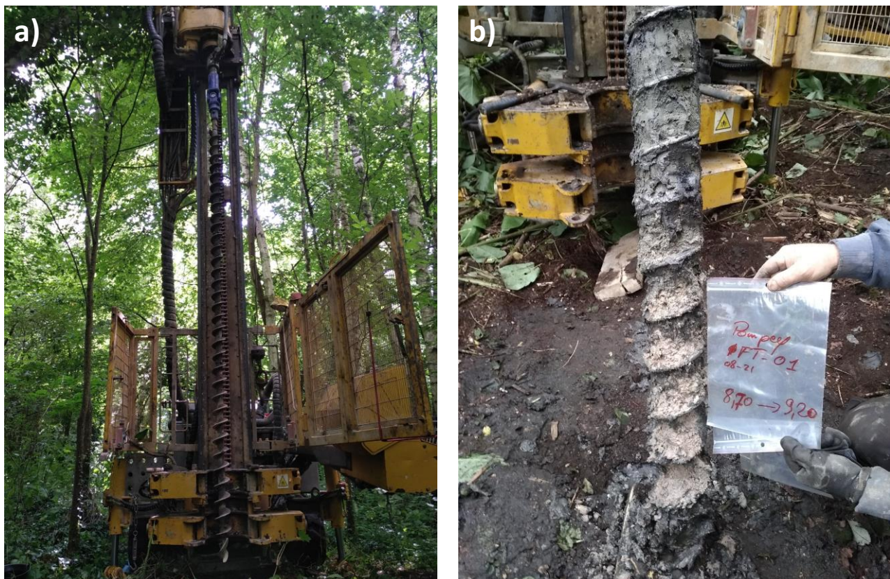
Figure 3 : a) Picture of the core drill in action in Pompey (08/2021); b) Zoom on the drilling rod with two different layers of soil.
